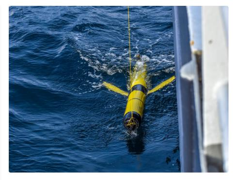
**Since November 2020**, the rechargeable Svinøy glider has been continuously deployed with servicing conducted during the **IMR Norwegian Sea** cruises that operate four or five times a year as part of a monitoring project that has been maintained in some form since the 1950s.
