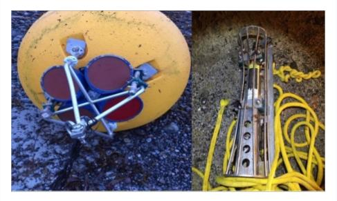
It was suspected that **high intensity fishing activity** in the area may have been responsible **for cutting** this top section of the mooring. On interrogation of the **CTD data** from the remaining part of the mooring, it became clear that the mooring was split on March 16th 2020.
