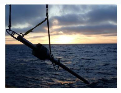
During the cruise we performed a **CTD survey** to measure and map the extent of the hydrothermal plume and its physical parameters.
