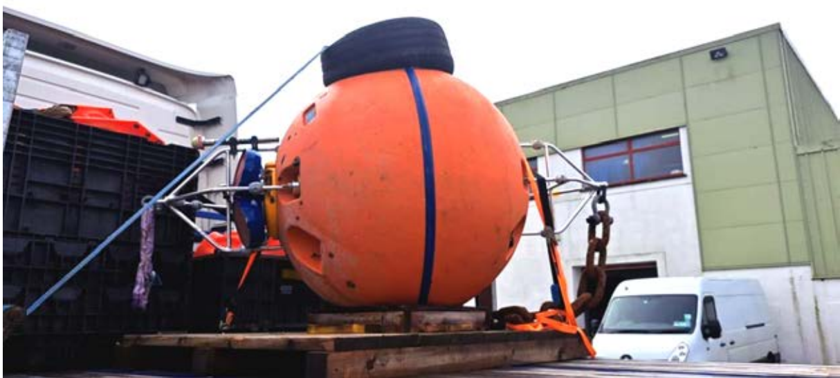
Figure 2 - ADCP mounted on a buoy in the Marine Institute of Ireland. Photo: Hugo Ferreira
