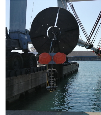
Scientific echosounder coupled to ADCP and multiple ultrasonic frequency recorders can quantify biomass and fish, or even plankton and/or krill, as environmental parameters vary.
