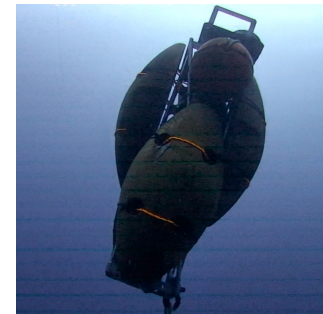
Scientific echosounder coupled to ADCP and multiple ultrasonic frequency recorders can quantify biomass and fish, or even plankton and/or krill, as environmental parameters vary.
